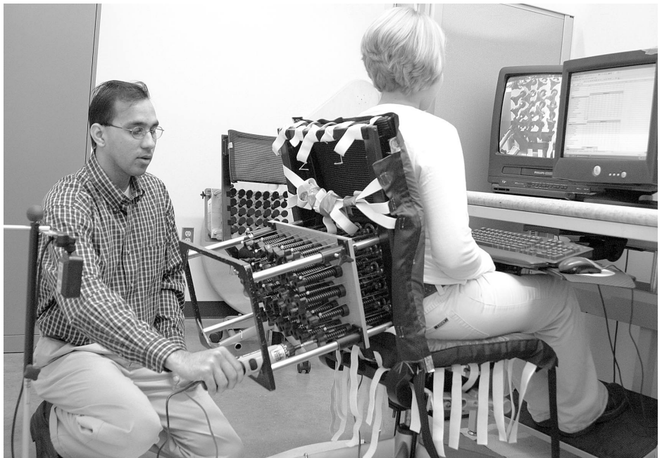
Figure 7.2 Illustration of laboratory setup used to conduct test-retest reliability assessments of user lumbar support asymmetries. (Photo courtesy of Haworth.)
